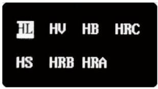
• Calibration: Short press the Enter button to enter the calibration interface, the screen prompts [Please measure the standard hardness block] and flashes, then you can measure the standard hardness block (single or multiple times). After measurement, the cursor moves to the actual value area, then press the or the press the
