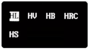
• Calibration: Short press the Enter button to enter the calibration interface, the screen prompts [Please measure the standard hardness block] and flashes, then you can measure the standard hardness block (single or multiple times). After measurement, the cursor moves to the actual value area, then press Enter or ▼ button to adjust the actual value to the standard value of the hardness block. Long
