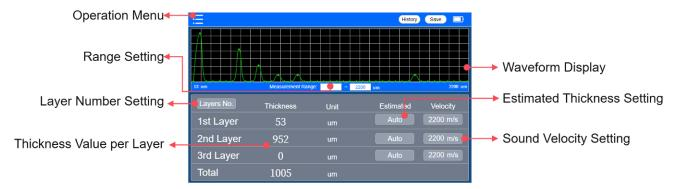
Thickness measurement results of 3 layers
