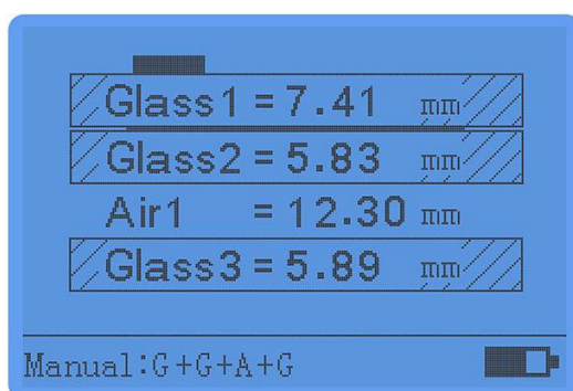
Laminated glass with one layer air
