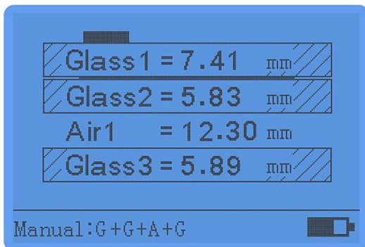
Laminated glass with one layer air
