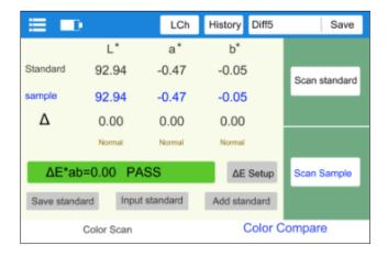
When the standard is measured or added and sample is measured, color difference between the two colors will be calculated with the following results:
