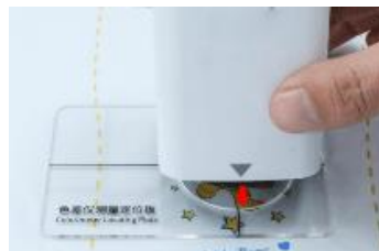
Place the meter on the positioning hole
