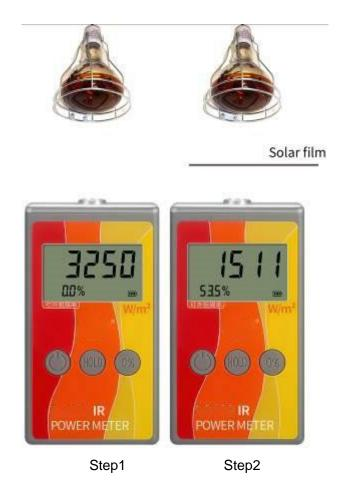
Figure 1: Measuring the infrared rejection rate of solar film
