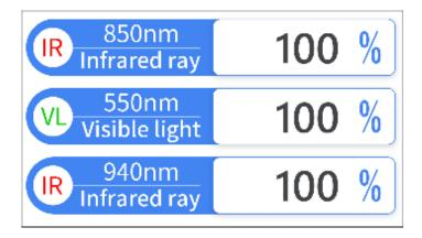
Select "550nm/850nm", the measurement interface display 550nm visible light transmittance, the 850nm infrared transmission;
